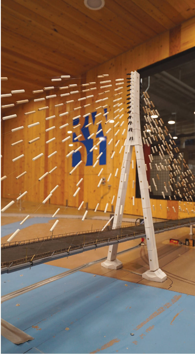
Gordie Howe International bridge model in RWDI's wind testing lab. Photo Courtesy of RWDI
